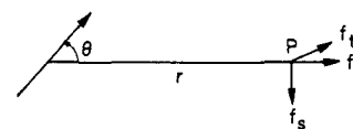
Figure 2. The components of the field at a point P due to an axially symmetric charge distribution.
